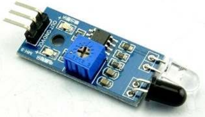
Gambar. 4. Infra Red Obstacle Avoidance FC-51 [Sumber : aliexpress.com]
